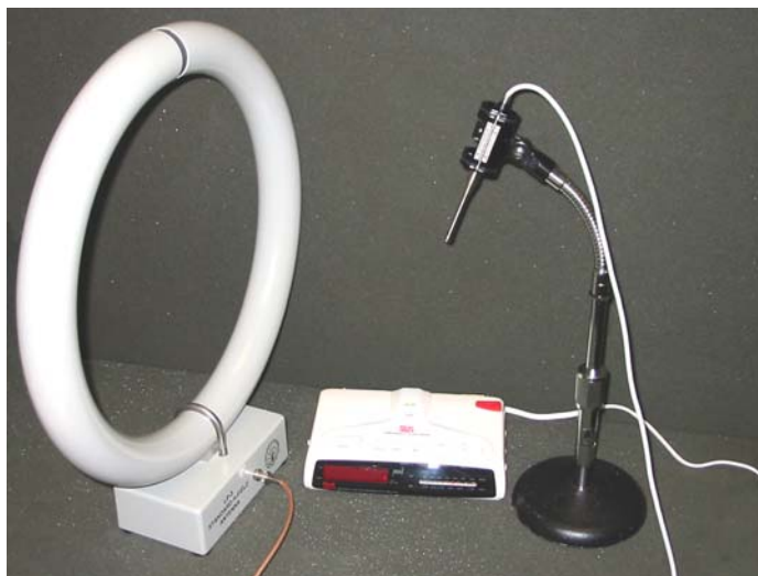
Figure 20 - Acoustic testing of Sima table radio with Bruel & Kjaer instrumentation microphone inside acoustic box of 1-ft. thick closed-cell foam. Magnetic field loop antenna also shown.
