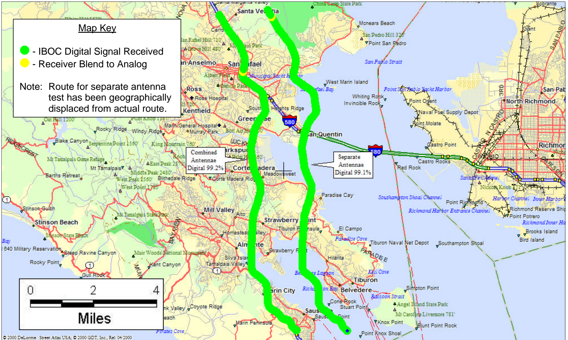
KDFC-FM, San Francisco – Separate vs. Combined Antenna - Northern Route
