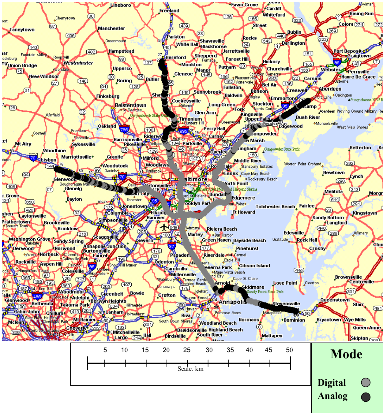
Figure 9 – WWIN Hybrid Performance (from NRSC Testing)
