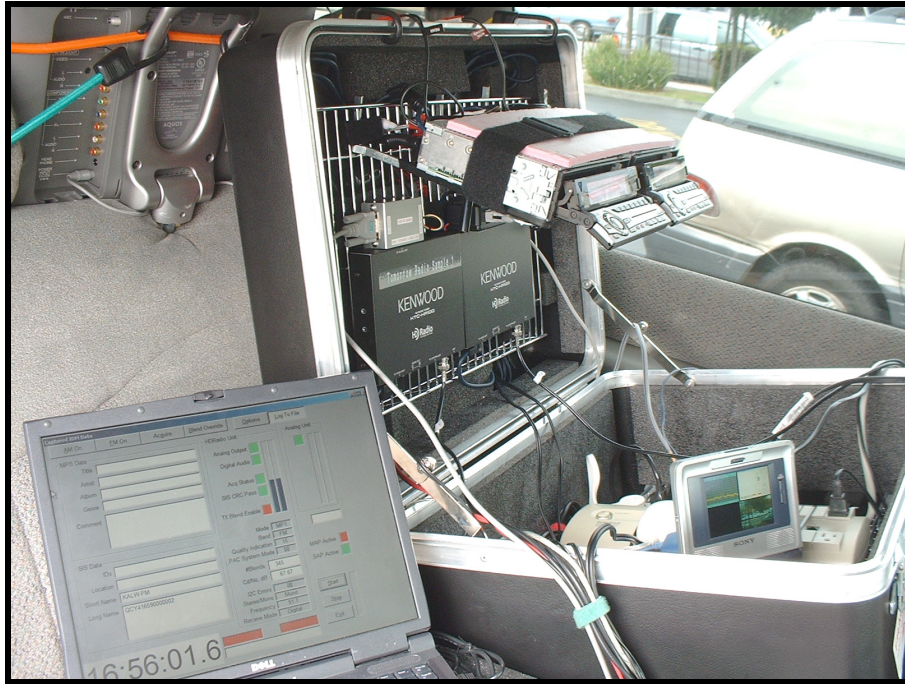
Portion of mobile test package showing test receivers and data gathering computer. (Courtesy Kenwood Corporation)
