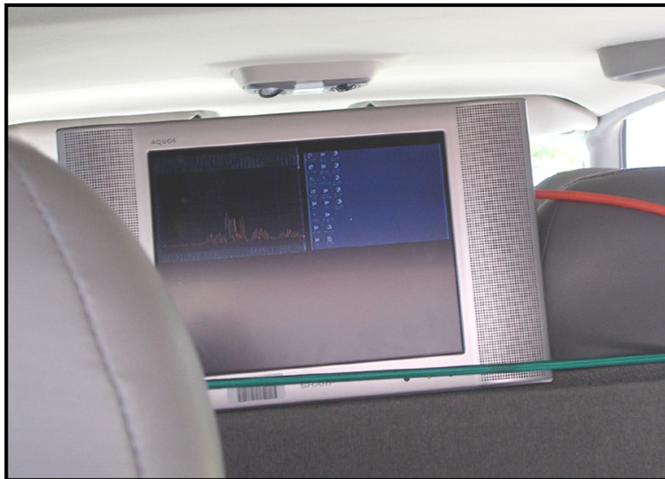
Video monitor in observer position used during original testing. Displayed spectrum, computer screen, forward camera image.
