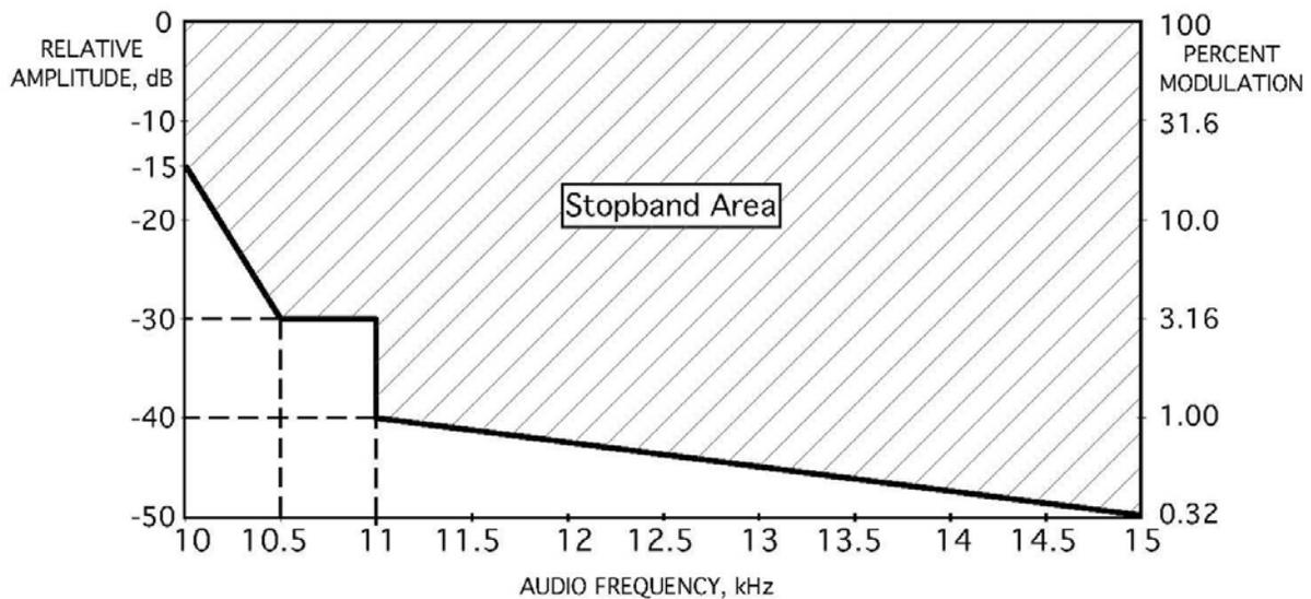
**Figure 4. NRSC Stopband Specification for Analog AM Transmission**
