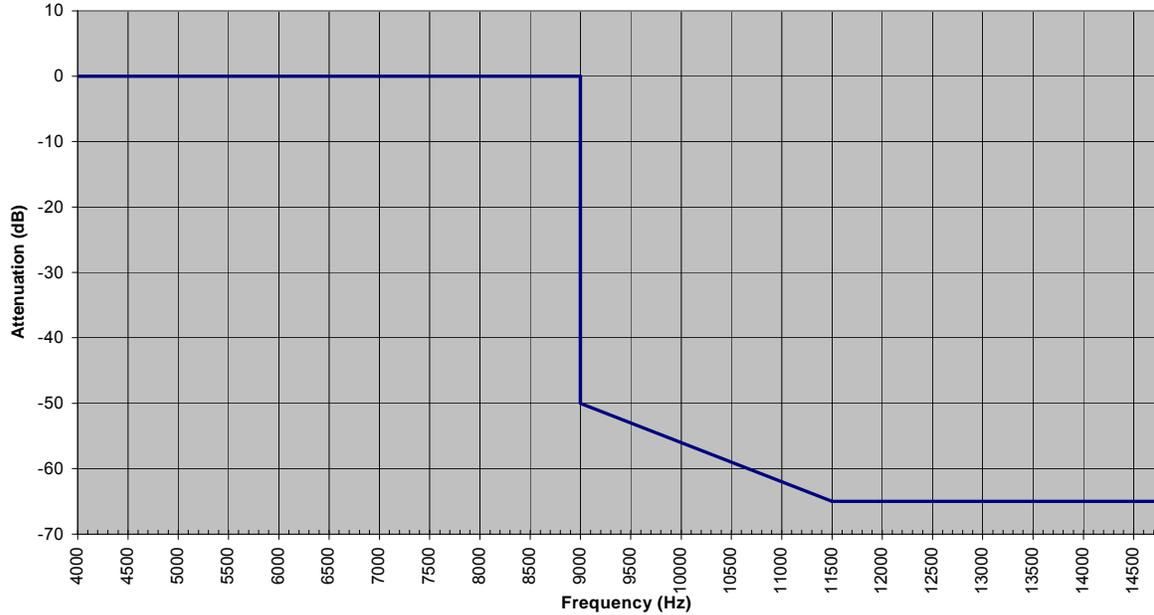
**Figure 6. NRSC Stopband Specification for 8 kHz Hybrid AM IBOC mode**
