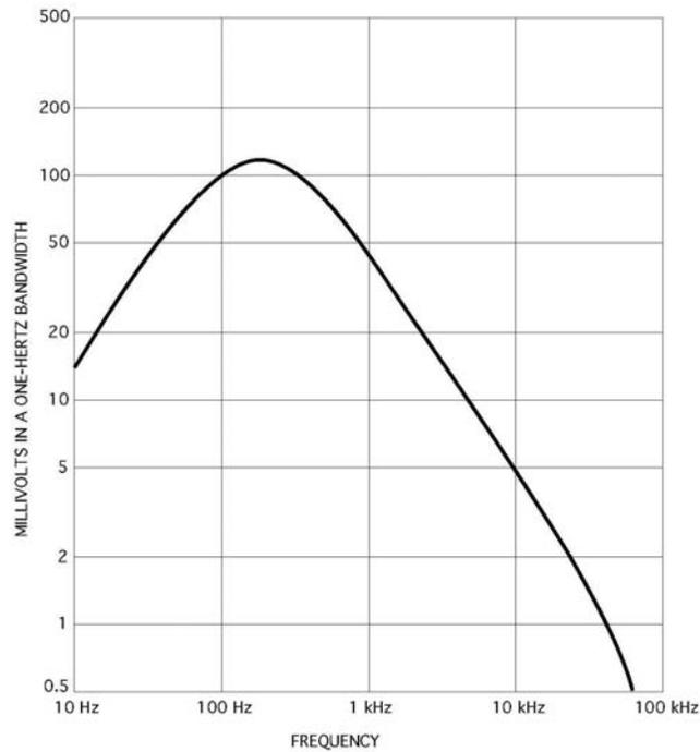
**Figure 7. Spectra of USASI Noise**
