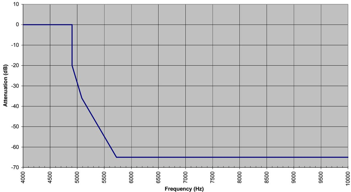
**Figure 5. NRSC Stopband Specification for 5 kHz Hybrid AM IBOC mode**
