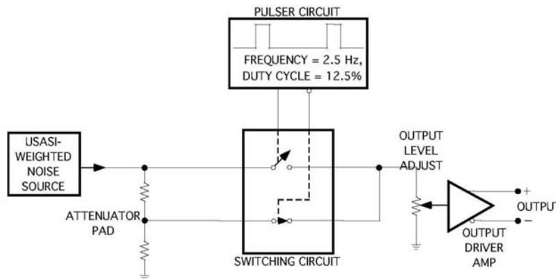
**Figure 8. Pulsed-USASI Noise Generator**
