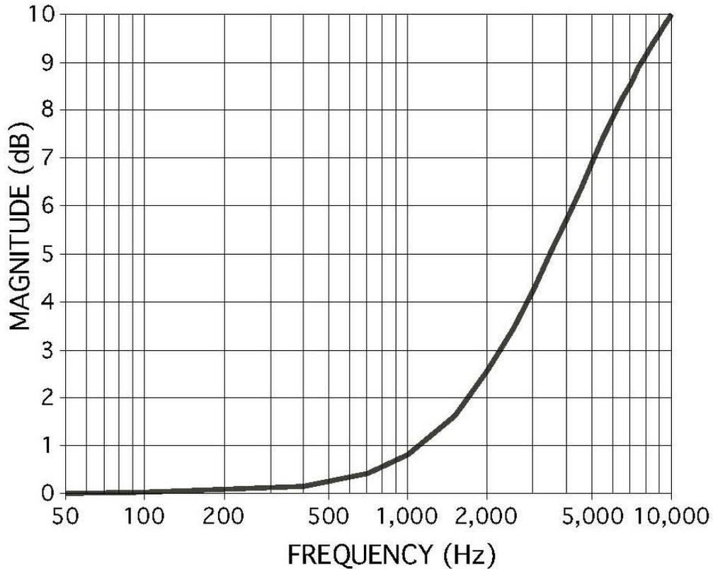
**Figure 1. Modified 75  $\mu$ s AM Standard Preemphasis Curve**
