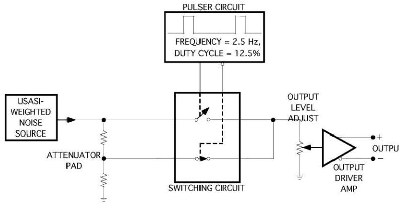
**Figure 6. Pulsed-USASI Noise Generator**
