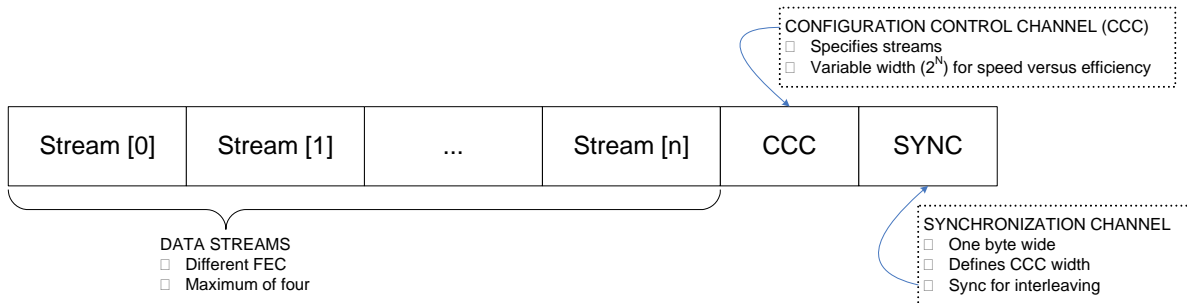
Figure 7-2: Fixed Bearer Channel Structure
