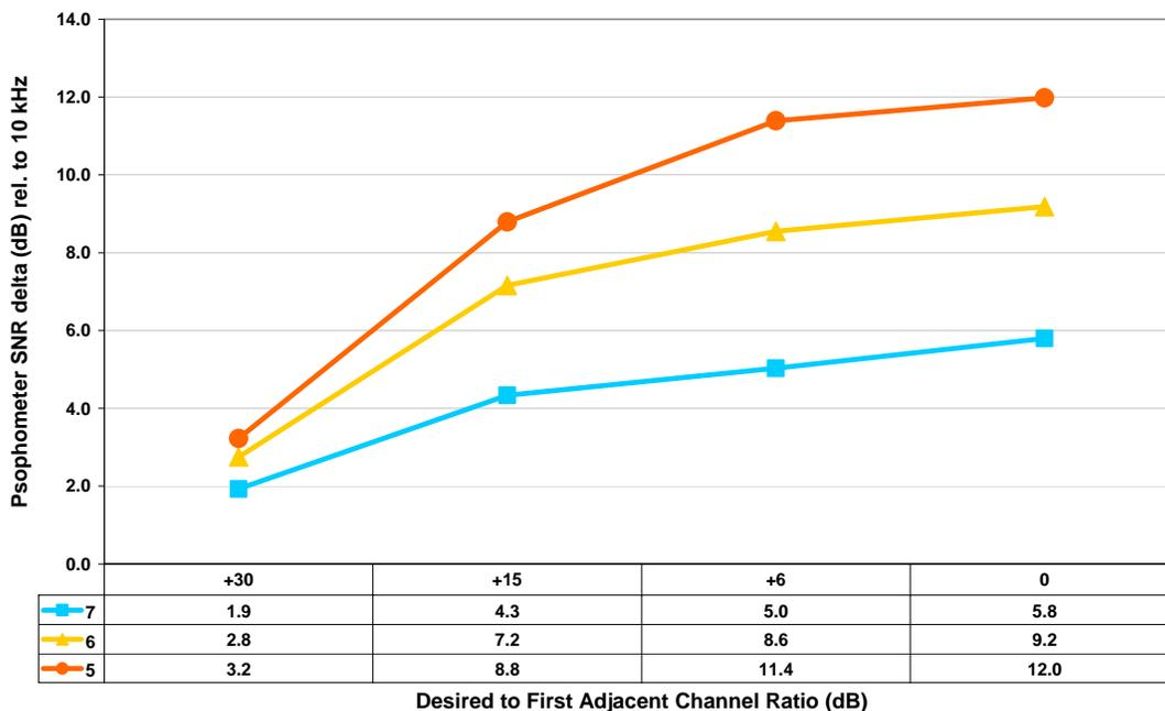
Figure 2. Effect Of transmission bandwidth on received SNR
