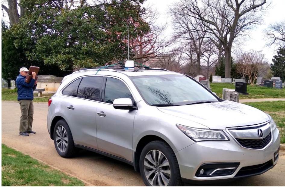
Figure 1. Measurement vehicle and antenna being calibrated with Potomac Instruments FIM-41 field strength meter.
