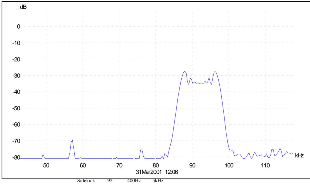
Plot of 67kHz and 92kHz SCA signals from Modulation Analyzer output
