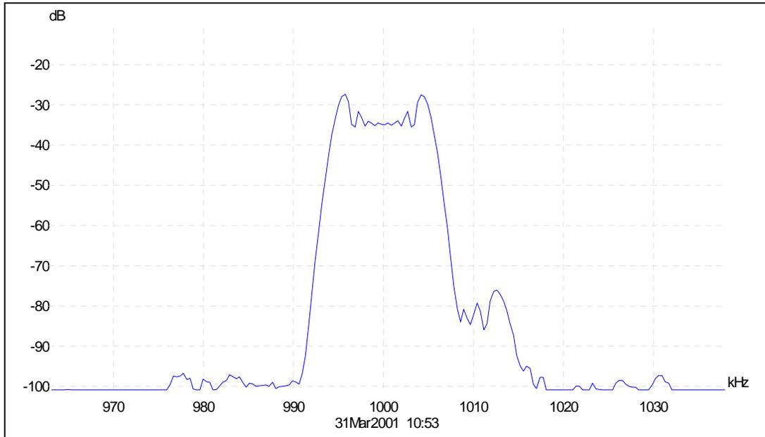
Plot of 67kHz SCA signal from Modulation Analyzer output
