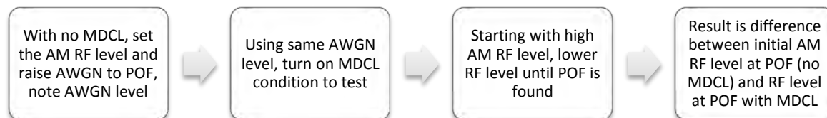
Figure 5 - Flowchart of basic measurement steps for MDCL compatibility tests
