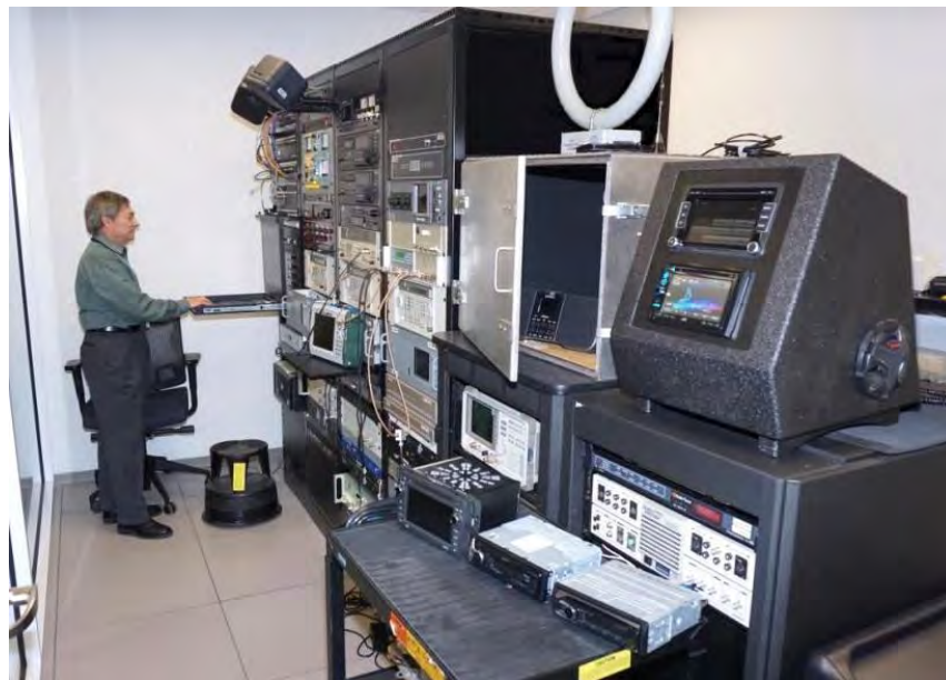
Figure 3 - View of RF Lab showing the car radios (3 on cart, 2 in black display cabinet) and the iBiquity/SPARC table radio (inside the shielded test enclosure with door ajar)
