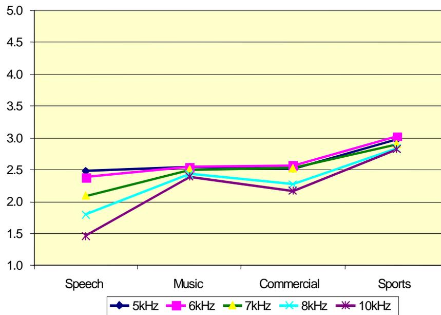
Given these results, a recommendation was made to include 7 kHz bandwidth as the 3rd bandwidth for consumer testing. This recommendation was based on two conclusions:
