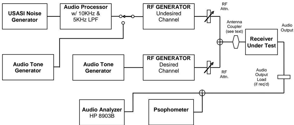
Measurements are listed in Appendix K for each receiver, titled Psophometer-Based Adjacent-Channel Interference. Each table reports the audio noise level, referenced to 1 kHz at 70 percent modulation, for interference at RF Desired-to-Undesired ratios of 30 dB, 15 dB, 6 dB (the minimum for FCC allocation purposes) and 0 dB.
