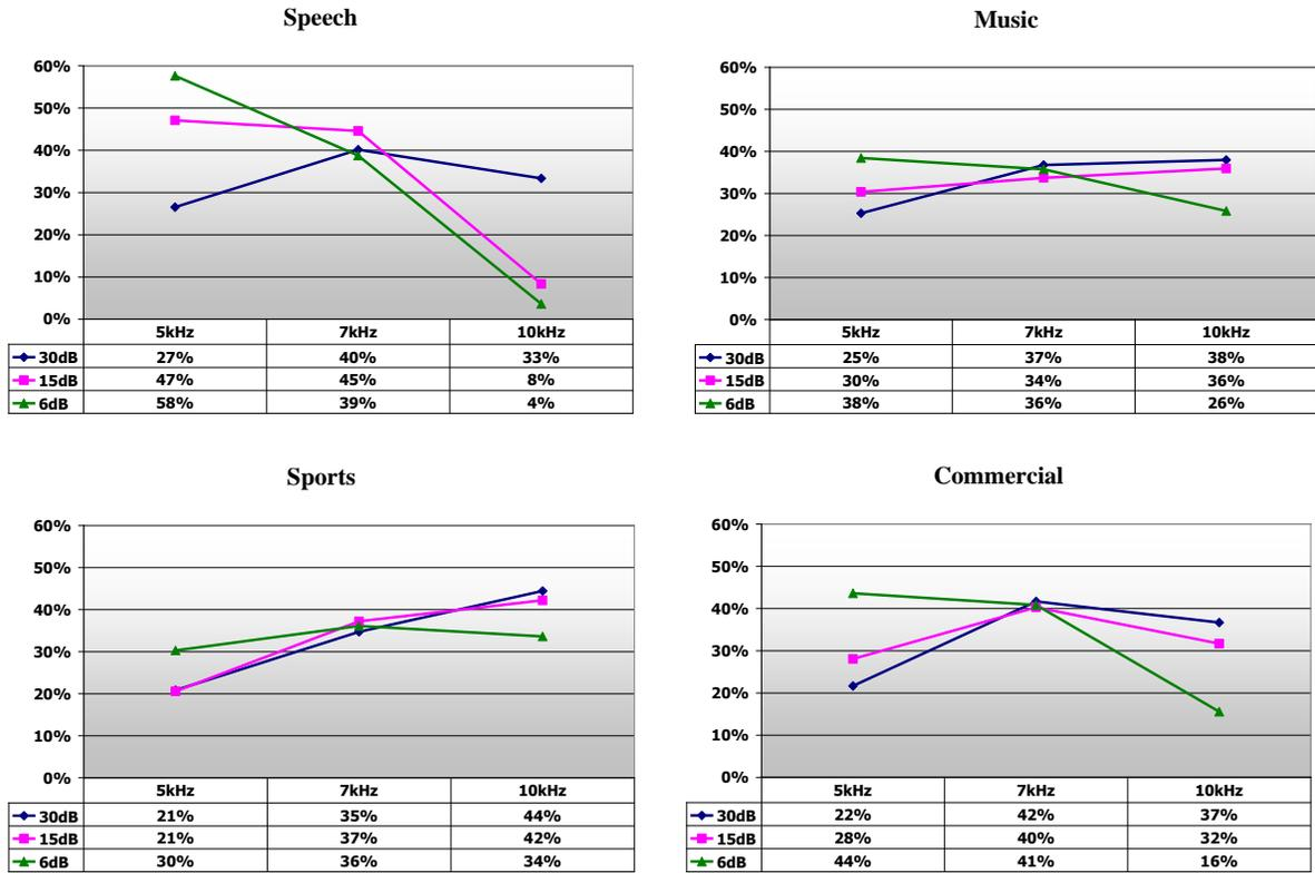
Figure 9. Percentages of listeners who picked one bandwidth over another, by genre, with no 1st-adjacent channel interference (30 dB), moderate 1st-adjacent channel interference (15 dB), and heavy 1st-adjacent channel interference (6 dB)
