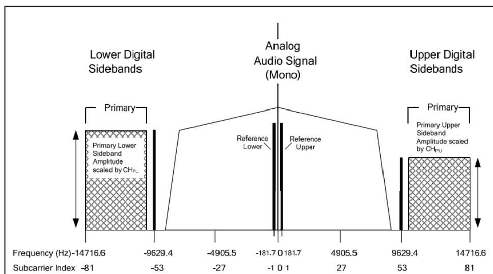
**Figure 12. Hybrid AM IBOC spectrum – reduced digital bandwidth configuration<sup>10</sup>**
