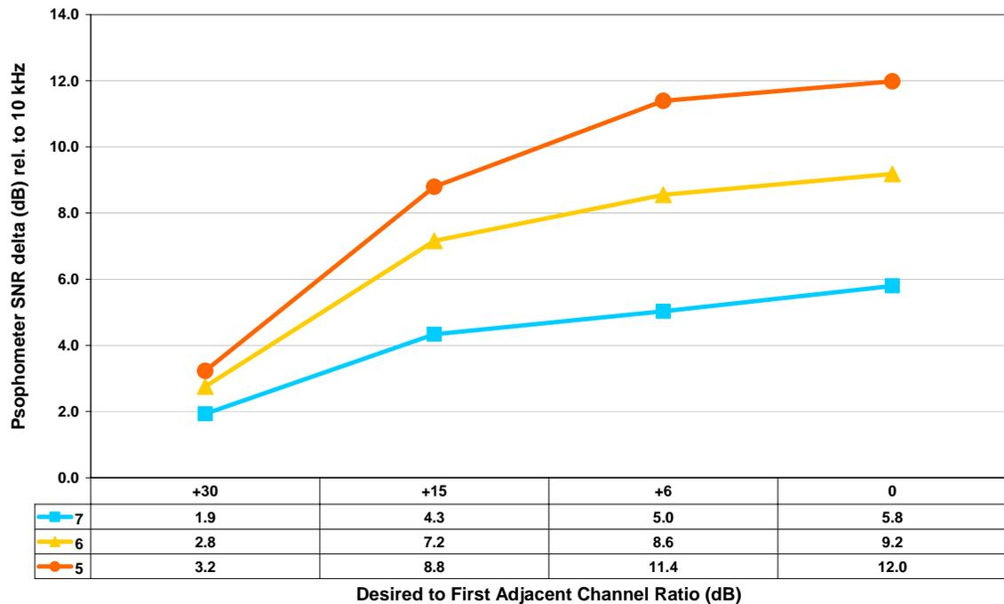
The upper and lower adjacent channel interference noise measurements of each receiver were averaged, and those receivers with WQP SNR measuring at least a 2 dB above
