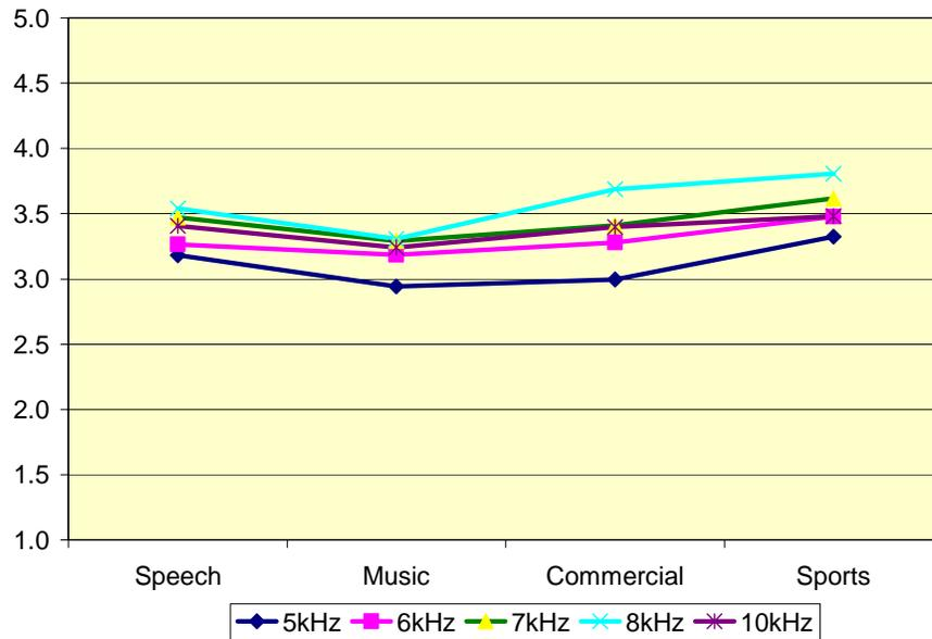
As shown in Figure 2 in the +15 dB condition, listeners generally preferred lower bandwidths to higher bandwidths, although, with the exception of speech, these differences were very small. In speech, they again showed a preference for lower bandwidths, particularly 7 kHz.
